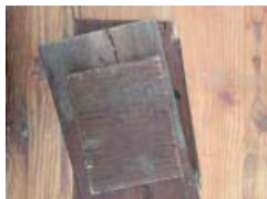
Fig. 33 - 40: 1. Collect offcuts, 2. Cut plugs, 3. Extract plugs, 4. Admire firewood, 5. Pre-drill and countersink fixings, 6. Glue holes, 7. Plug holes, 8. Sand and oil plugs.
